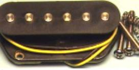
OL® -yksikelainen TC-tyylinen ala mikrofoni. Mukana ruuvit ja jouset. Single coil TC -style rear pickup. Screws and springs included. DC -resistance 7.1k, inductance 5.9 H. Resonant frequency typically 2.9 kHz. Relative gain @ resonant frequency typically 3 dB. Wires ( yellow /black). Polepiece spacing 53.5mm. Order code: **MICT-535 15.00€**
